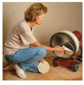
so the sanding heads are exposed by laying the machine's handle on the floor. The sanding pads have "hook & loop" backs, so just press them into place on the sanding pads. Stand the machine up and you are ready to go.
